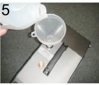
Remove filler cap and slowly add smoke oil to the Phantom. Check the sight glass and do not overfill.
