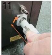
To use remote push in an twist to the right The remote switch then duplicates the function of the Black Smoke Switch on the machine. If either switch is on, the Phantom will produce smoke.
