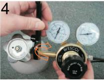
Attach regulator to CO2 cylinder and tighten with spanner supplied
