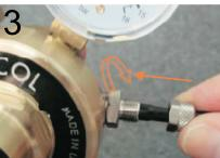
Tighten nut with spanner
