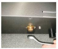
If sending the machine via a courier we always recommend oil is removed from the machine to prevent spillage, and a drain is fitted to assist this
